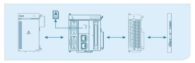
Snap-in installation and detachable terminal blocks, implementing quick installation
